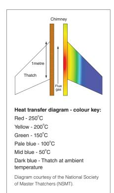
Over a period of time the temperature of the thatch chimney interface can become critical (approx. 200°C) and lead to a chain of events that cause a thatch fire.
